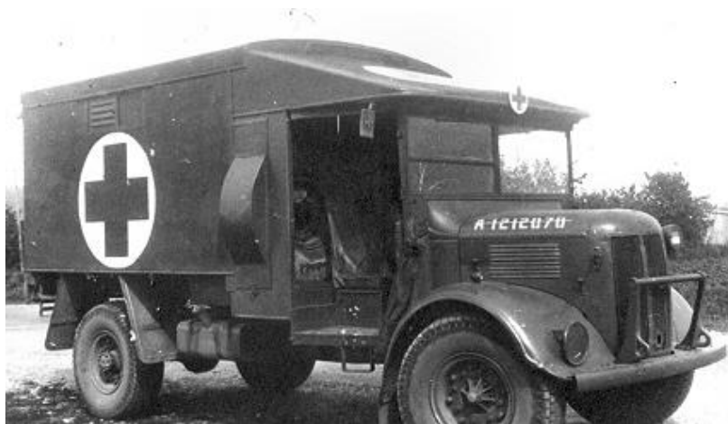
Fig 7.2b - Over 13,000 ‘Katies’ were built for the war and despite the temperamental gearbox they were known for their reliability and sturdy construction 42 . The top speed was around 50 mph The Mann Egerton was also fitted to Bedford and Morris chassis.
