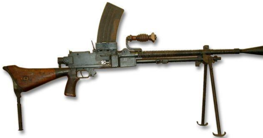
Fig 4.8b – The Type 99 LMG was a marked improvement on its predecessor. This image shows the gun fitted with the 30 round magazine and the butt rest deployed.
