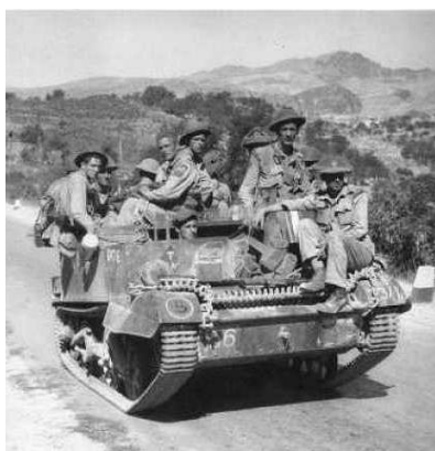
Fig 5.12a - A Mk.I Universal carrier in service in Italy. It is carrying ten men with weapons and equipment.
