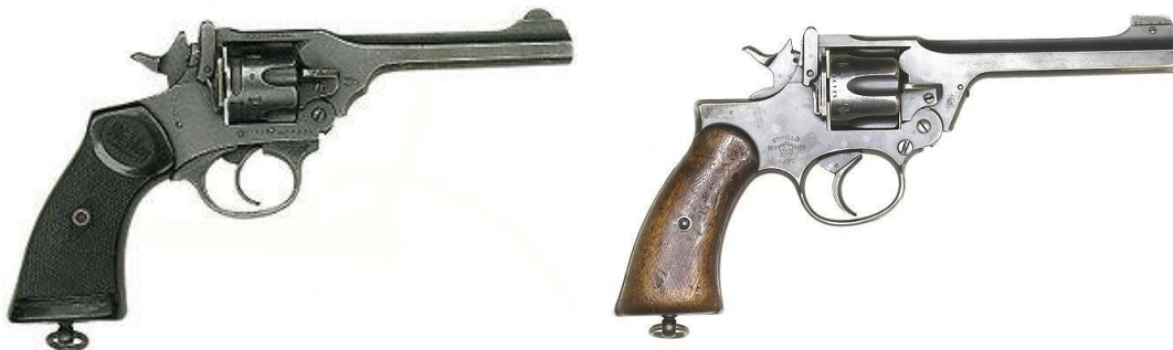
Fig 12 a & b – the Webley Mk IV .38/200 revolver on the left and the Enfield equivalent on the right. The similarities between the Webley and Enfield designs were so obvious that Webley sued the British Ministry of Supply and won. Both weapons used .38/200 ammunition
