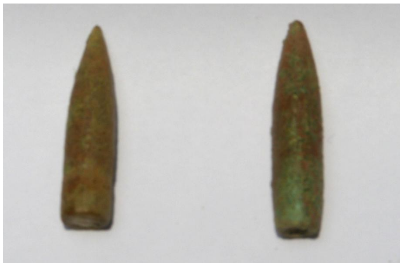
Fig 20 - What was notable amongst the bullet collection was a distinct difference in appearance between .303 ball and incendiary rounds. The latter tend to have a smaller crimped base as seen in the example of the right.
