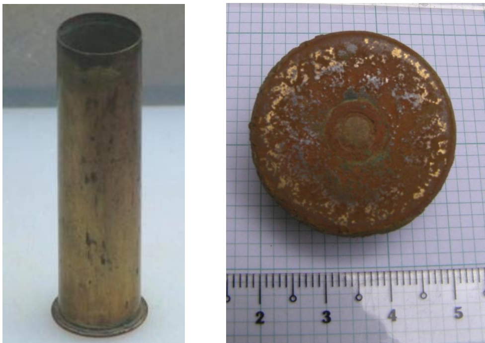
Fig- 13 a& b Item 11/12/06 is thought to be the base of a 30mm shell probably for the Webley & Scott flare gun, an example of which is shown on the left.
