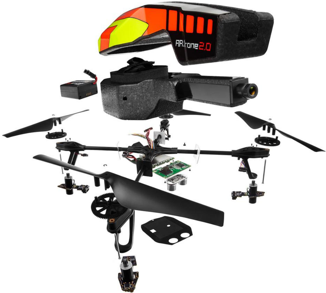
Fig 19 – A construction diagram showing the component parts of the AR Drone 2.0. The machine has proven a cheap and usable platform for aerial photography. Solving the problem of a downward facing camera would increase its usefulness in the field.
