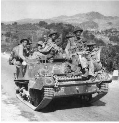
Fig 12a - A Mk.I Universal carrier in service in Italy. It is carrying ten men with weapons and equipment.
