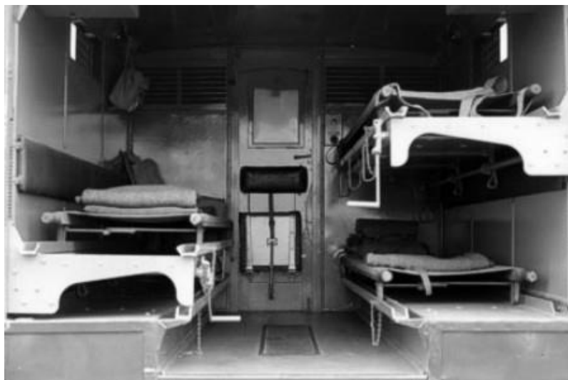
Fig 3a - The rear body, built by Mann Egerton, could take 10 casualties sitting or 4 stretcher cases.
