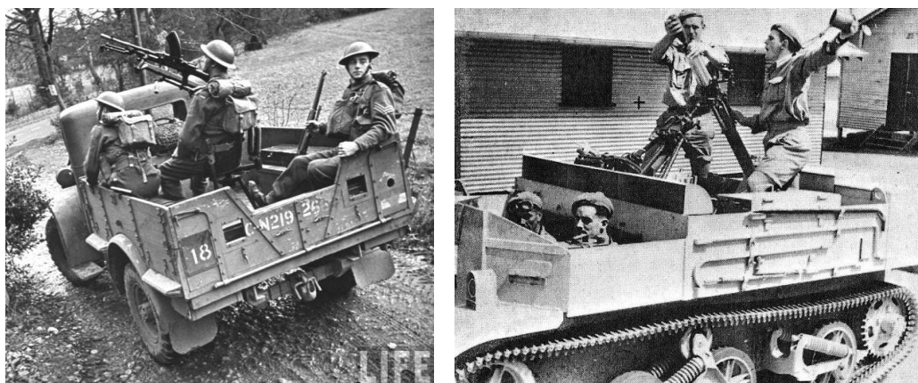
Fig 2a A 15cwt truck fitted out in the AA role with a single bren mounted on the flatbed pictured during a training exercise in the UK
