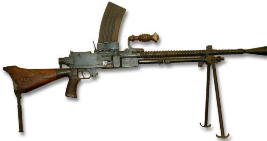
Fig 23b – The Type 99 LMG was a marked improvement on its predecessor. This image shows the gun fitted with the 30 round magazine and the butt rest deployed.
