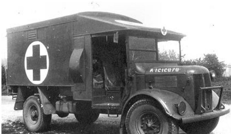
Fig 3b - Over 13,000 'Katies' were built for the war and despite the temperamental gearbox. They were known for their reliability and sturdy construction 36 . The top speed was around 50 mph The Mann Egerton was also fitted to Bedford and Morris chassis.
