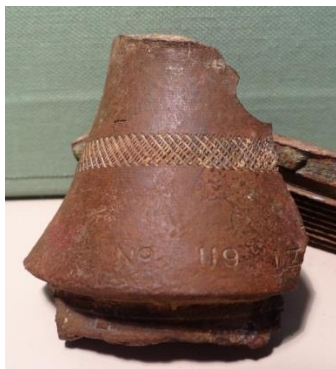
Fig 32a, b and c, - a, No. 119 mortar fuse fragment (see data sheet in Fig, 20 b), b, No. 43 mortar fuse fragment (both a & b are British fuse, located on the surface on the NW slope, c, What appears to be Japanese mortar fuse fragment, stamped with the Japanese symbol for No.8, (八), discovered in P.A. 3
