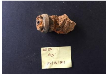
Fig 31 - Possible British mortar fuse No. 119 - AMI/C, striker cover and safety catch.
