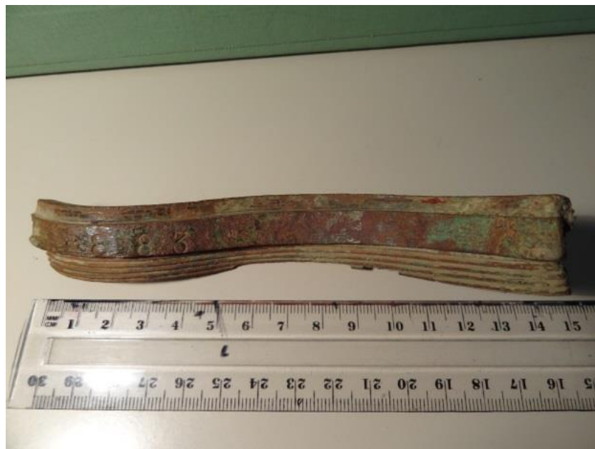
Fig 33 – Appears to be a shell or Bomb casing joining band, stamped with the number 883 on the rim. Located, P.A. 3.
