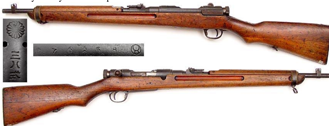
Fig 30 - Japanese Arisaka Type 38 rifle, 6.5 mm calibre rifles.
