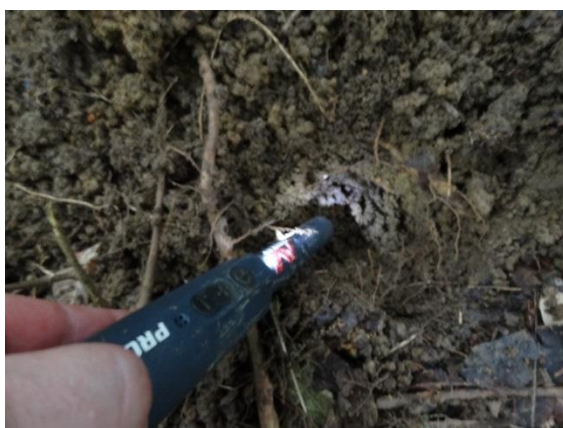
Fig 13a & b – Picture a, is locating the aforementioned round with the use of a MINELAB PRO-FIND 25. Picture b, is the discovery of the find.
